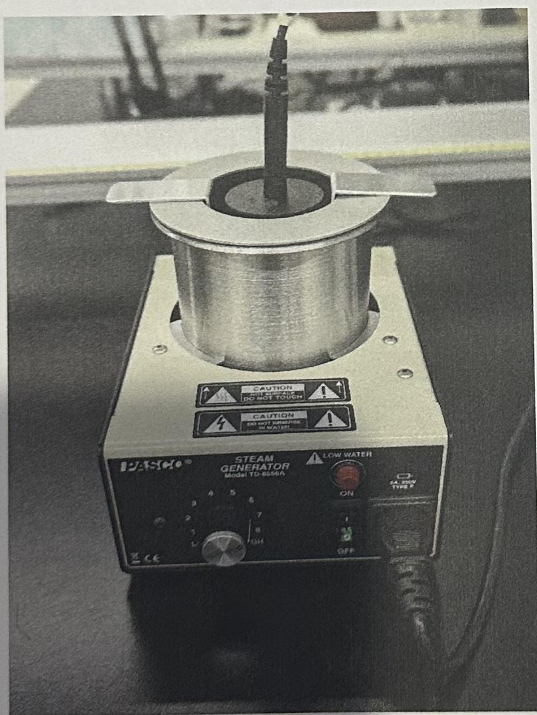
FIGURE 1. 3: The aluminum cylinder + cradle is placed in the steam generator to heat the water inside the cylinder. Temperature Probe 2 is threaded through the rubber stopper to measure the water's temperature.
